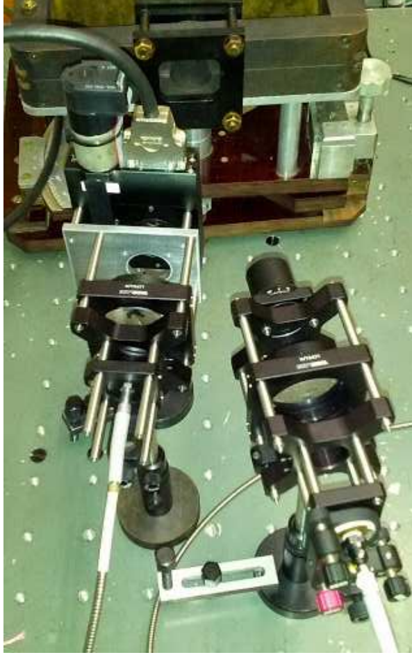
Figure 6.4: Picture of magneto-optical spectrometer with rotating analyzer.
