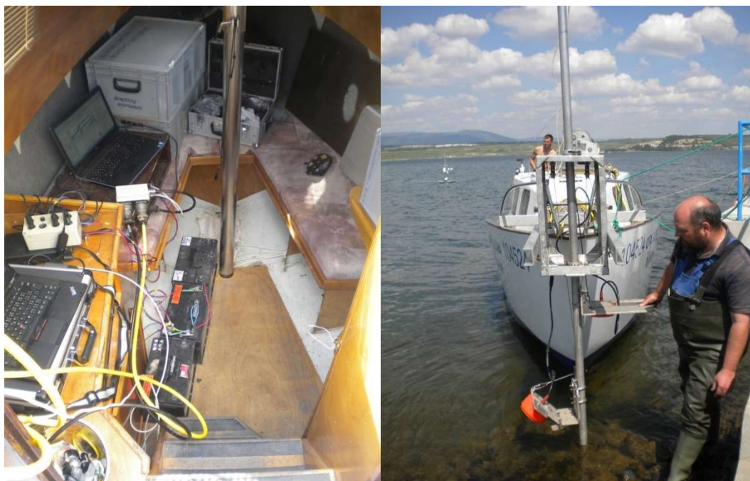
Obr. 5: Simrad EK60 split beam (foto autor)
