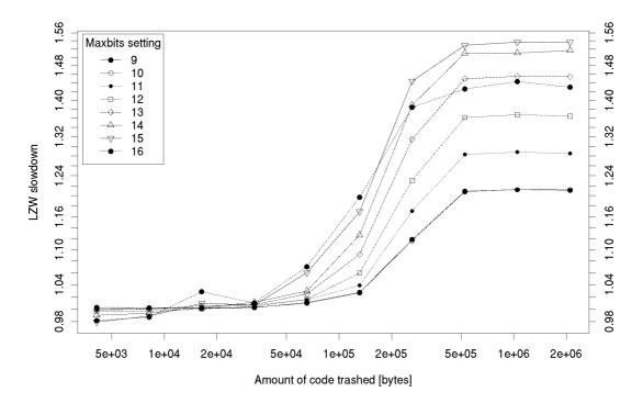
Figure 3.21: Effect of code cache trashing on the LZW performance on Platform 1, various dictionary sizes, trashing after each 8 KB of input data
