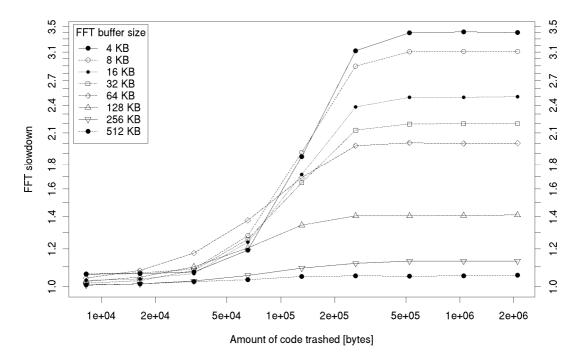
Figure 3.12: Effect of code cache trashing on the FFTW in-place transformation performance on Platform 2
