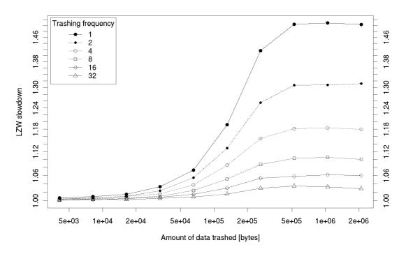
Figure 3.19: Effect of data cache trashing on the LZW performance on Platform 2, various trashing frequency, maxbits set to 9
