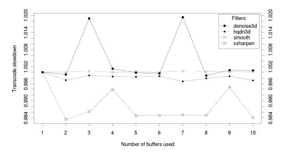
*Figure 3.23:* Effect of the number of buffers used in Transcode with fixed synchronization on its performance with one filter on Platform 1
