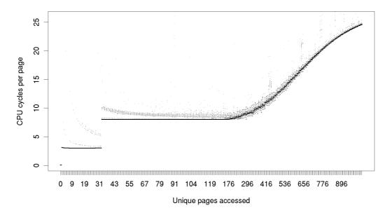
Figure 3.1: The effect of TLB trashing on Platform 1
