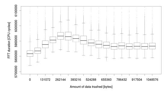
*Figure 3.13:* Unusual effect of data cache trashing improving the simple FFT performance with a 256 KB buffer
