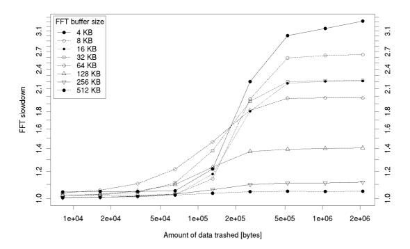
*Figure 3.10:* Effect of data cache trashing on the FFTW in-place transformation performance on Platform 2
