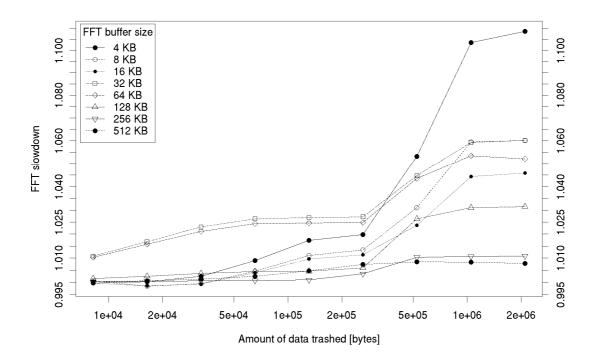
Figure 3.7: Effect of data cache trashing on the simple FFT implementation performance on Platform 1
