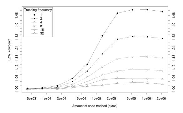
*Figure 3.20:* Effect of code cache trashing on the LZW performance on Platform 2, various trashing frequency, maxbits set to 9
