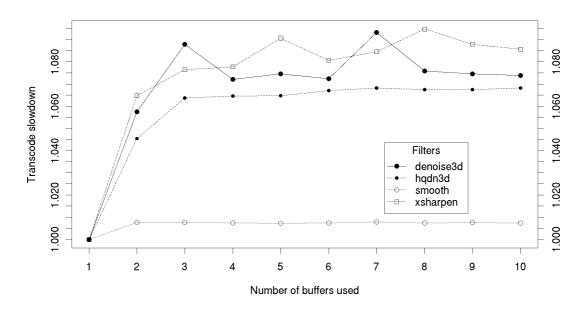
*Figure 3.22:* Effect of the number of buffers used in Transcode on its performance with one filter on Platform 1
