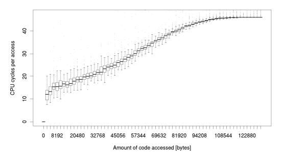
Figure 3.6: The L1 code cache miss latency on Platform 2 with random access
