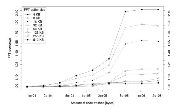
*Figure 3.11:* Effect of code cache trashing on the FFTW in-place transformation performance on Platform 1
