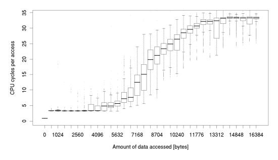
Figure 3.5: The L1 data cache miss latency on Platform 2 with random access
