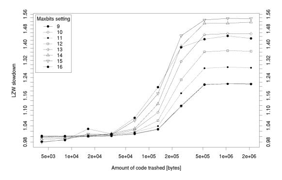
Figure 3.17: Effect of data cache trashing on the LZW performance on Platform 1, various dictionary sizes, trashing after each 8 KB of input data
