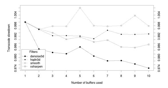
*Figure 3.24:* Effect of the number of buffers used in Transcode with modified synchronization on its performance with one filter on Platform 2
