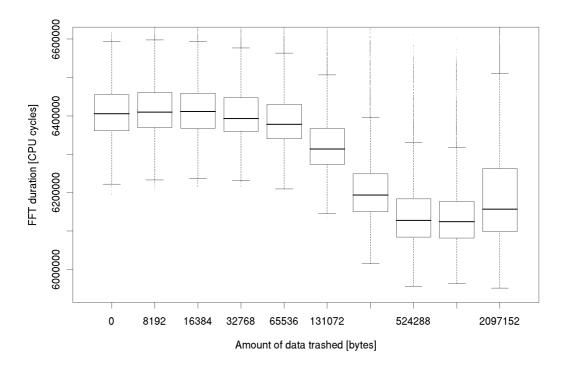
Figure 3.16: Unusual effect of data cache trashing improving performance of FFTW with two separate 512KB buffers on Platform 2
