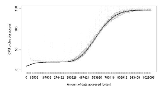
Figure 3.3: The L1 and L2 data cache miss latencies (including the L1 TLB miss latency) on Platform 1 with random access
