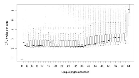
Figure 3.2: The effect of TLB trashing on Platform 2
