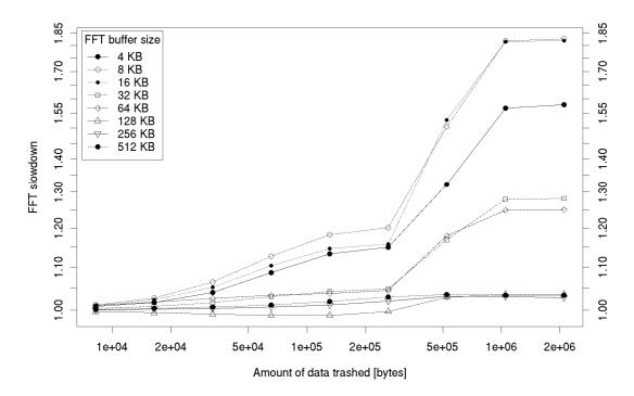
*Figure 3.9:* Effect of data cache trashing on the FFTW in-place transformation performance on Platform 1
