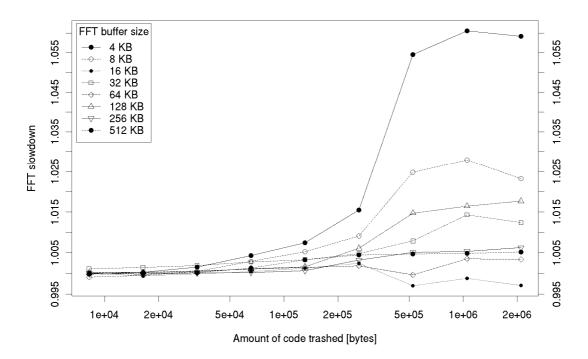
*Figure 3.8:* Effect of code cache trashing on the simple FFT implementation performance on *Platform 1*
