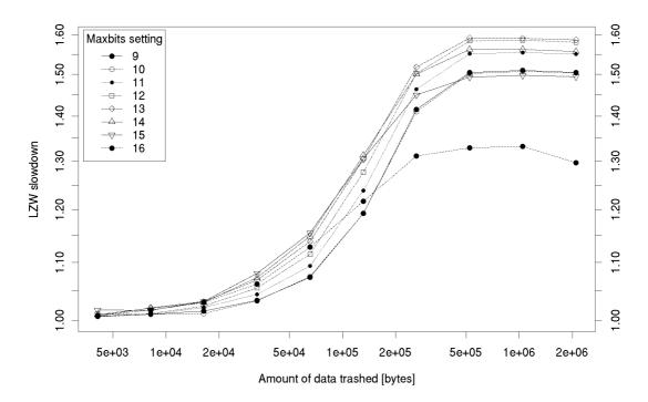
Figure 3.18: Effect of data cache trashing on the LZW performance on Platform 2, various dictionary sizes, trashing after each 8 KB of input data
