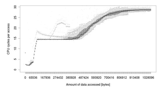
Figure 3.4: The L1 and L2 data cache miss latencies on Platform 1 with linear access
