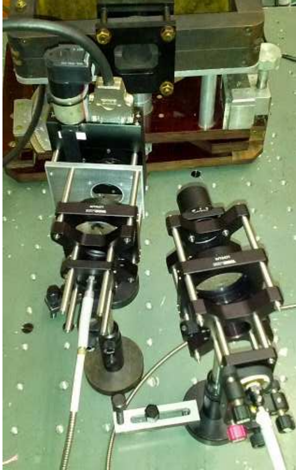
Figure 6.4: Picture of magneto-optical spectrometer with rotating analyzer.
