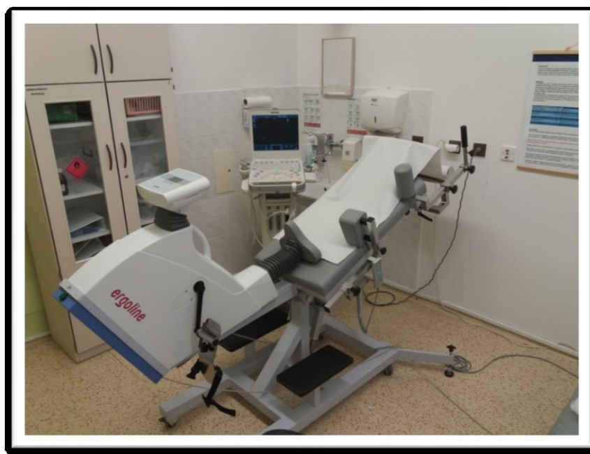
Figure 0. Tilt-able bicycle ergometer. Patient may be tilted on the left side and backwards in the position, which is almost identical with the common one, for the standard transthoracic echocardiography, resulting in almost all patients in reasonable image acquisition.
