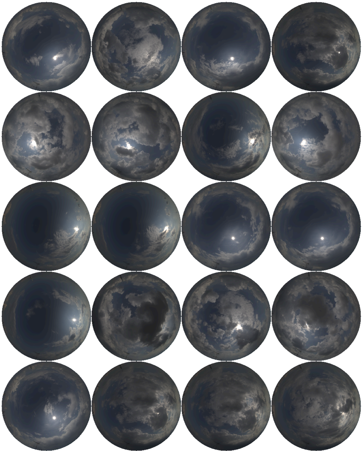
Figure 5.2: Sample images from the small dataset of 714 images captured on 2019-07-14 from the Prague rooftop. We picked a sunny day with rapidly moving cumulus clouds, so there is large variation in the cloud positions, but the appearance of the clouds is very consistent.
