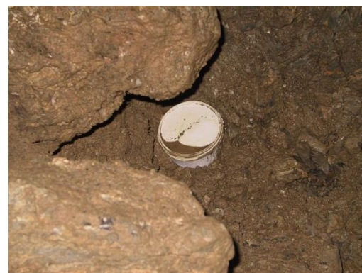
Definitely a wrong location for a RAMARN detector
