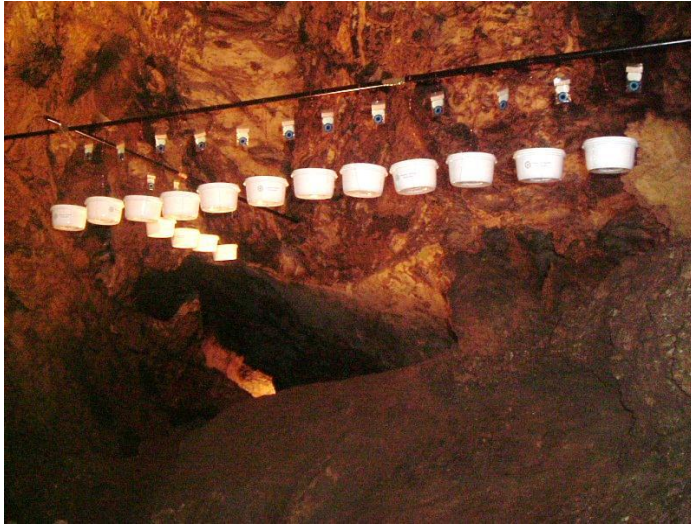
Figure 32 Integral detector test arrangement in the Božkov Dolomite Caves
