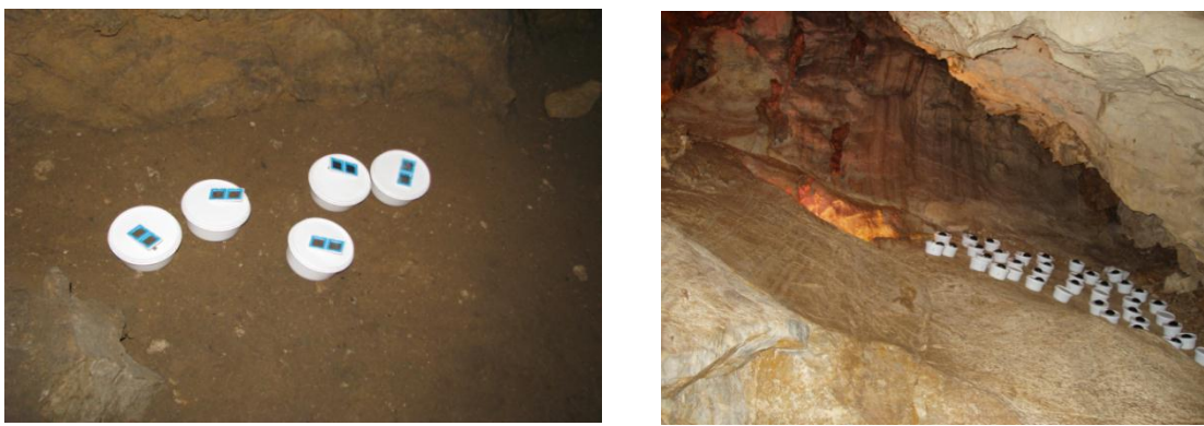
Figure 34 Inter-comparative measurements in the Bozkov Dolomite Caves (RAMARN and DRPS/DTPS detectors; RAMARN and CR39 detectors in black plastic boxes)
