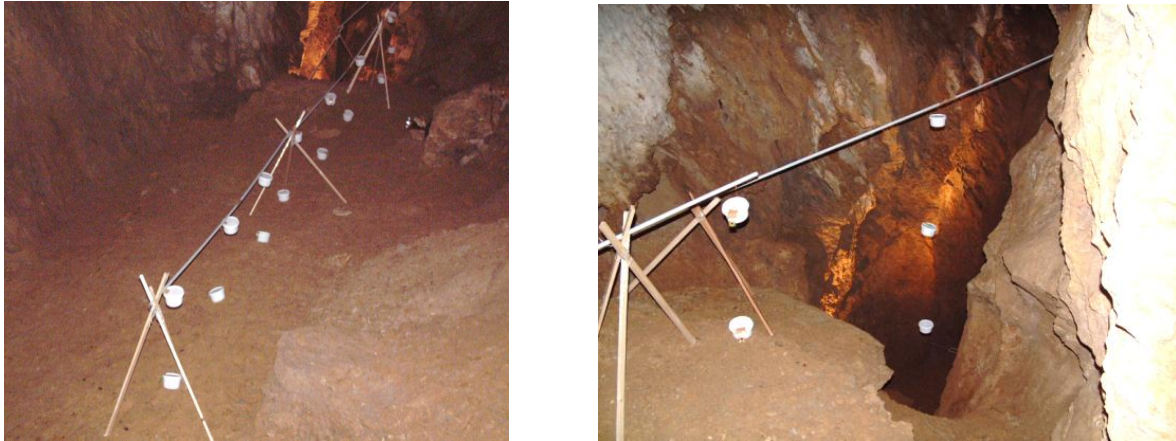
Figure 30 Placement of RAMARN and SSNTD detectors in pairs for comparison in the Zbrašov Aragonite Caves ; the main test in the Gallaš's Dome
