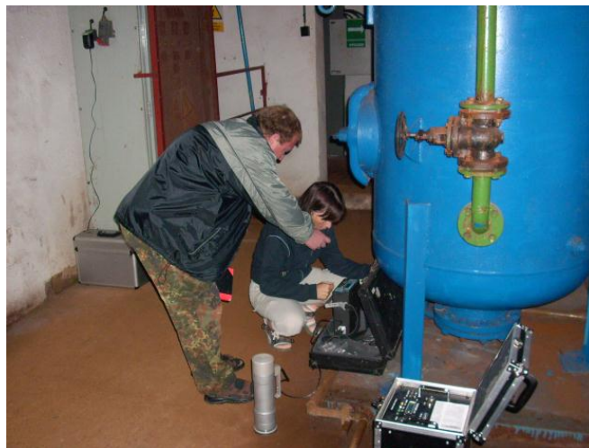
Measurements in the Hanička underground Fortress. RADONIC01, NB3201 devices.
