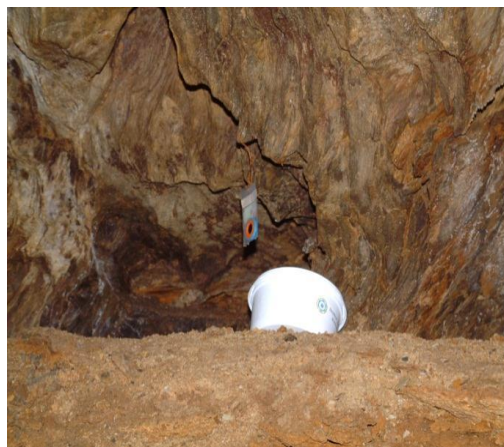
Figure 31 Placement of detectors in pairs along the visitor's path
