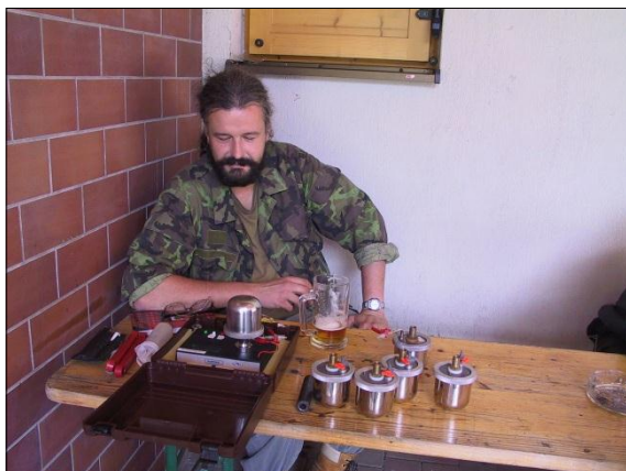
IK-250 ionization chamber in measurement position
