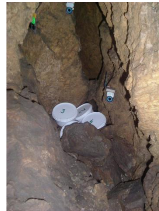
Figure 32 Integral detector test arrangement in the Božkov Dolomite Caves
