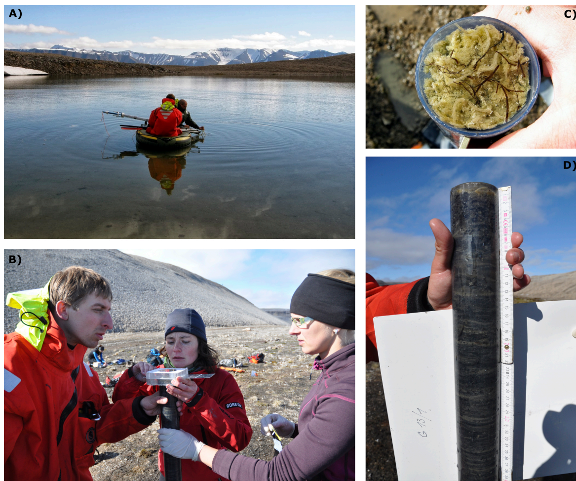
Figure 9.2 Coring Garmaksla sediments using Kajak gravity corer and rubber boat (A); cutting the profile in 1cm steps (B); bottom of the lake (top of the core) with green algae and plant macroremains (C); the upper part of core G13/1 with distinct lamination (D). Coring and subsampling was performed analogously in northeastern Norway. Photos A, B, D taken by the author, C by Dan Vondrák.
