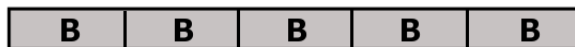
Figure 2.1: A chromosome representing an individual with five genes ( N=5 ). B marks a B -bit wide binary block.
