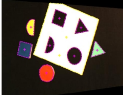
Figure 5.3: The segmentation result produced by this algorithm. Distinct classes are labeled by different colors. The crosses in the image give the representative points of segmented objects.
