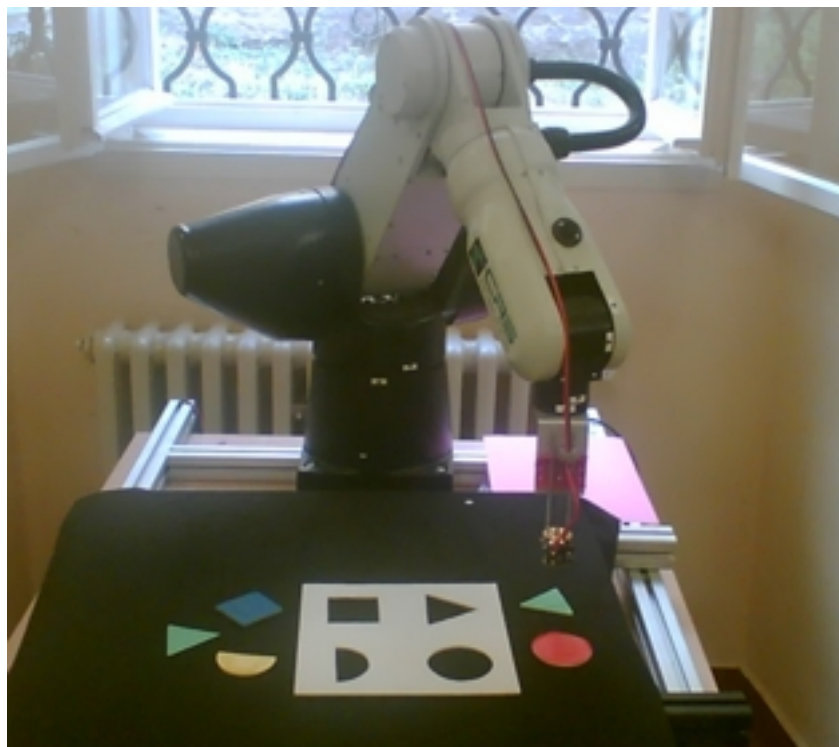
Figure 1.2: The industrial robot CRS A-465 with six degrees of freedom with installed electromagnet and with the puzzle.
