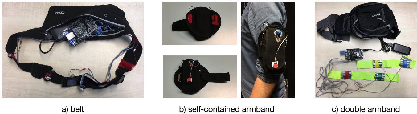
Figure 2: The MHWs prototypes involved during the technology demonstrations: a) a belt equipped with four motors; b) a self-contained armband equipped with two motors and two buttons; c) a pair of armbands both equipped with two motors.
