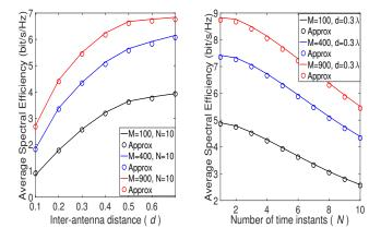
Fig. 3. Average SE v.s. a) inter-antenna distance and b) number of time instants for K = 5,  $p_p = p_u = 0$  dB and  $p_r = 10$  dB.
