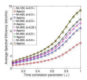
Fig. 4. Average SE v.s. time correlation parameter for K = 5, N = 10,  $p_p = p_u = 0$  dB and  $p_r = 10$  dB.
