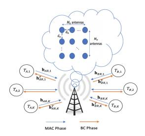
Fig. 1. Multi-pair D2D two-way half-duplex DF relaying system with spaceconstrained massive MIMO.
