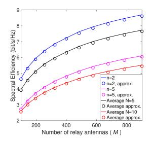
Fig. 2. SE v.s. number of relay antennas for K = 5,  $d = 0.3\lambda$ ,  $p_p = p_u = 0$  dB and  $p_r = 10$  dB.
