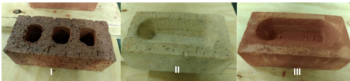
Figure 1: Brick types: I. more porous/less dense brick with a rough surface finish (perforated); II. a less porous/more dense brick with a smooth surface finish (frogged) and III. a more porous/less dense brick with a smooth finish (frogged)
