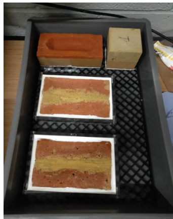
Figure 7: 3 different types of specimen during absorption test
