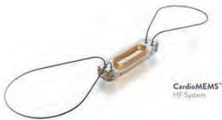
Fig. 3 CardioMEMS HF system, consisting of the pulmonary artery pressure sensor ( a ) and the patient electronics system ( b ) used to take daily pressure readings Courtesy of Abbott, Inc. to provide the illustrations
