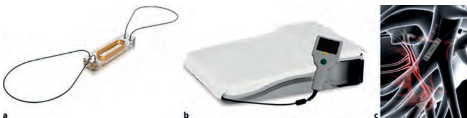
Fig. 2 a The CardioMEMS sensor (with permission of Abbott Inc.). b The CardioMEMS HF system patient unit including antenna (with permission of Abbott Inc.). c Location of the CardioMEMS sensor in the left pulmonary artery (with permission of Abbott Inc.)
