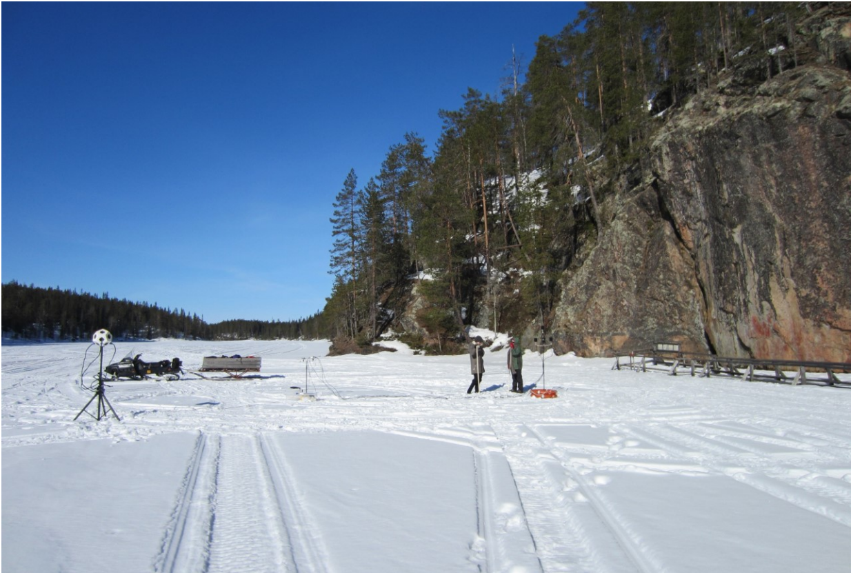
Fig. 3 Recording setup on ice in front of the Väräkallio cliff. From left: the dodecahedron loudspeaker, the snow mobile with a sledge, the recording and playback devices, researchers Tiina Äikäs and Annu Mikkonen, the tetrahedron microphone array, the spectator pier and the painted cliff. Photograph: Riitta Rainio
