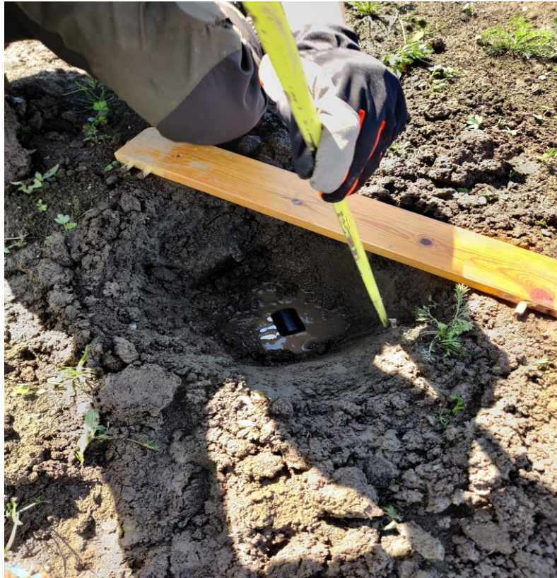
Figure 5. Measuring the depth of the pit in which the sensors were placed.
