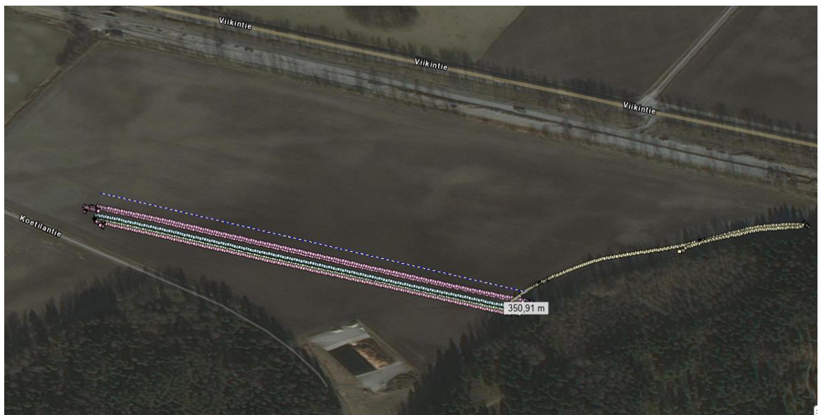
Figure 14. Map of the follow-up trace recorded with GNSS connected to Raspberry Pi.
