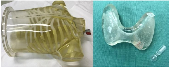
Figure 1. Thorax phantom, the thyroid gland and spherical phantom mimicking parathyroid adenoma. Images are not in scale.
