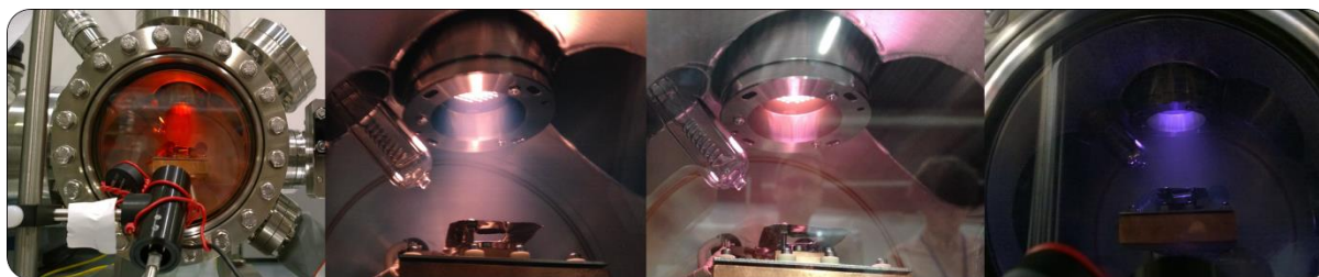
Fig. 3. Photographs of commissioning plasmas. From left to right these are neon, helium, air and argon. The divergence of the ion beam can be observed.
