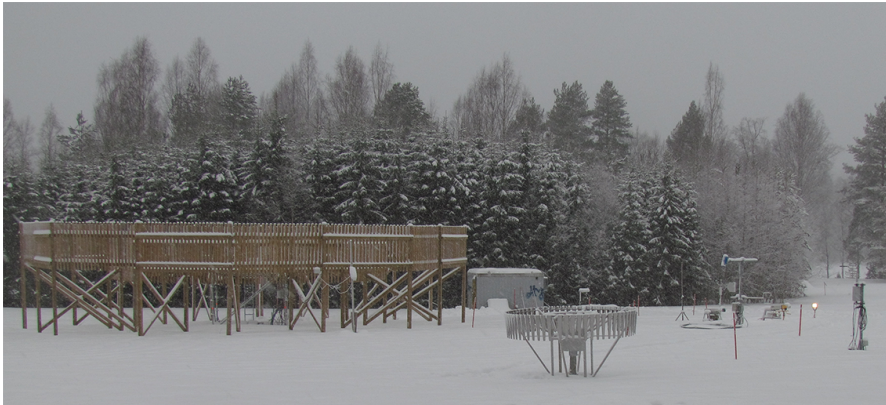
Figure 1. Snow precipitation instruments on the measurement field in Hyytiälä. The Pluvio 2 200 is inside the wind protection on a platform and the PIP lamp can be seen at right on the ground. The view of the picture is to southwest and the distance from the platform to the treeline behind is approximately 20 m.
