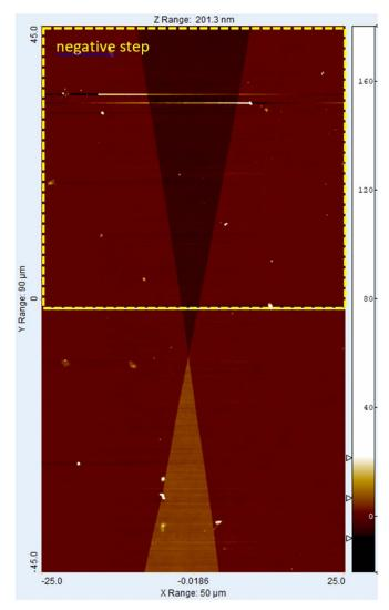
Figure 3. Height map of NanoStar sample measured using the AFM.
