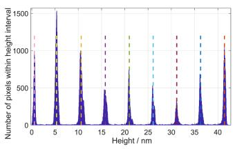
**Figure 6.** Histogram of heights measured from the NanoRuler using CSI, with the average height of each step indicated with dashed lines.
