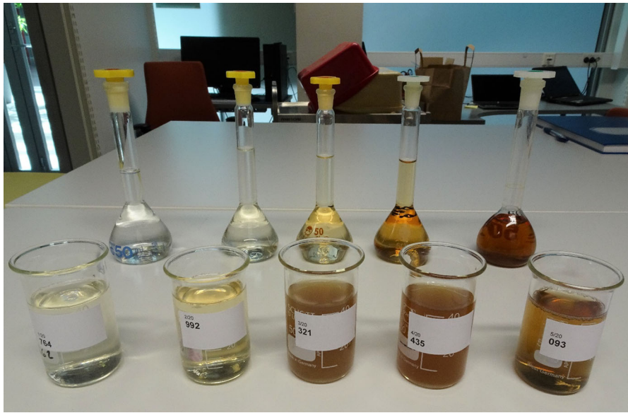
Fig. 1 Evaluation of the intensity of the brown color (experiment I). Samples in the front, reference samples behind. Samples from left to right: 0.5 wt% GA, eGX, sGGM, sGX, and
