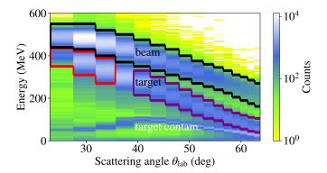
FIG. 1. The spectrum of the double-sided silicon strip detector shows the energy of the scattered heavy particles as a function of the scattering angle with respect to the beam axis (laboratory frame). Three different types of particles, heavy target, light target (contamination), and beam particles, are clearly separated. The gate for targetike particles is divided in single-hit (red) and double-hit (purple) events.
