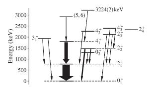
FIG. 3. The partial level scheme of  $^{140}Nd$ . The widths of the transitions correspond to the observed intensities. The  $2^+_1 \rightarrow 0^+_1$  transition width is scaled down by a factor of 5 for visibility.
