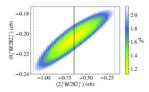
FIG. 4.  $\chi^2$ -surface distribution with respect to the diagonal and transitional matrix elements of the  $2_3^+$  state. The dashed gray lines indicate the limits of the diagonal matrix element of the  $2_1^+$  state, which is applied to the  $2_3^+$  state.
