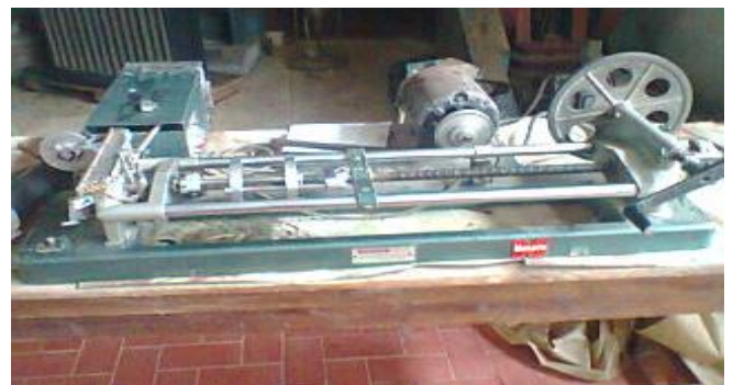
Figure 4: Monsanto Hardness Testing machine
