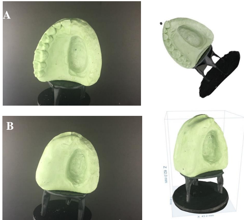
A: Example of an ideal image with resultant 3D model (Sample 2). B: Example of an ideal image with resultant 3D model (Sample 18)
