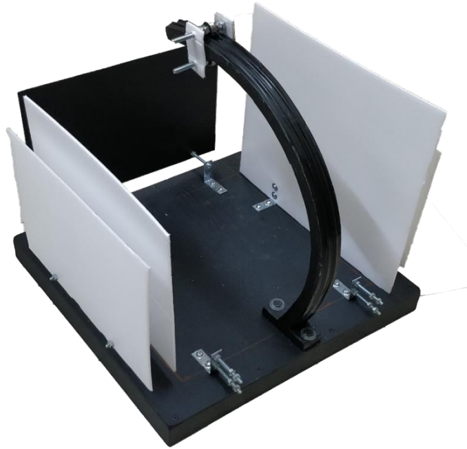
Figure 3.7 Corrugated white diffuser sheets with white LEDs and black focusing sheet
