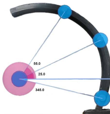
Figure 3.6 The angles on the arc where magnetic sleeve stops were placed
