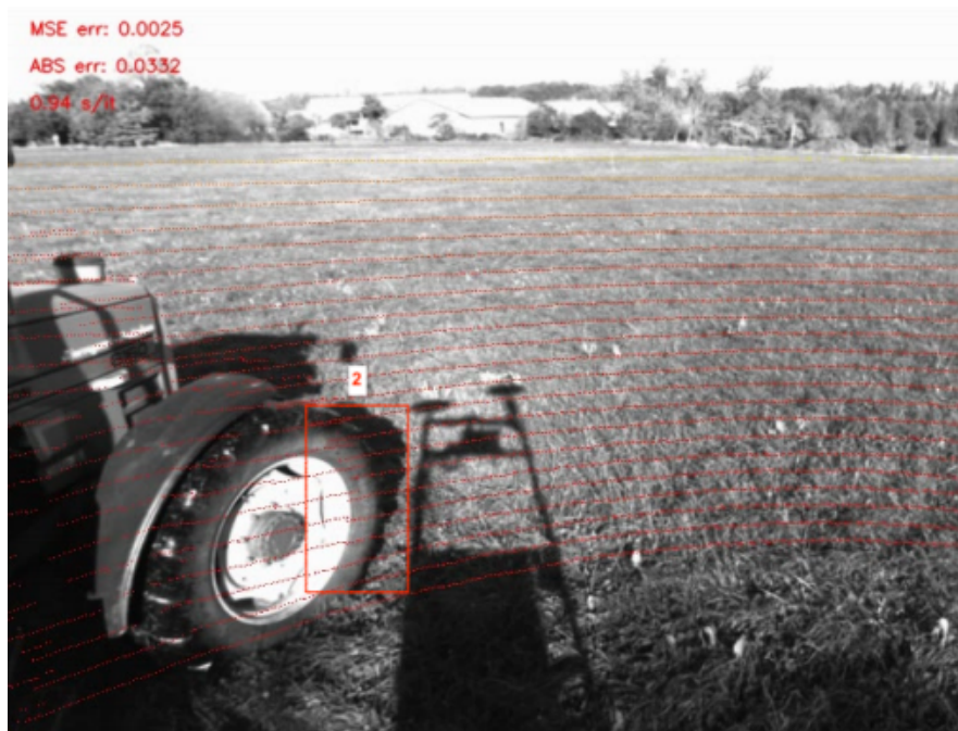
Figure 6. Example of LiDAR reprojected on the image. Note that a small error in the calibration will result in strong error on the estimated depth (see Square 2). We processed the error w.r.t. the depth obtained by stereo-vision.
