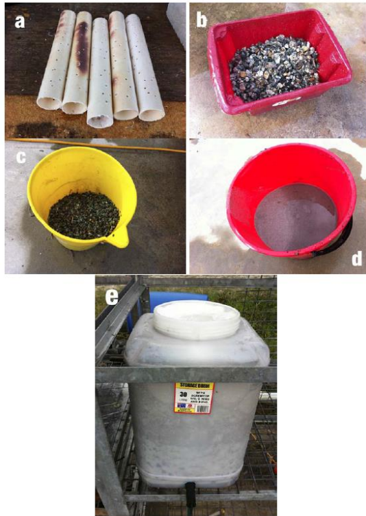
Figure 7. The setup of the sand filter. The materials layered into the drum from bottom to top include: a) Perforated pipes, b) Coarse Gravel, c) Medium Gravel, d) Coarse Sand, e) Non-absorbent cotton wool placed as the top layer in the drum (Ayre, 2013).
