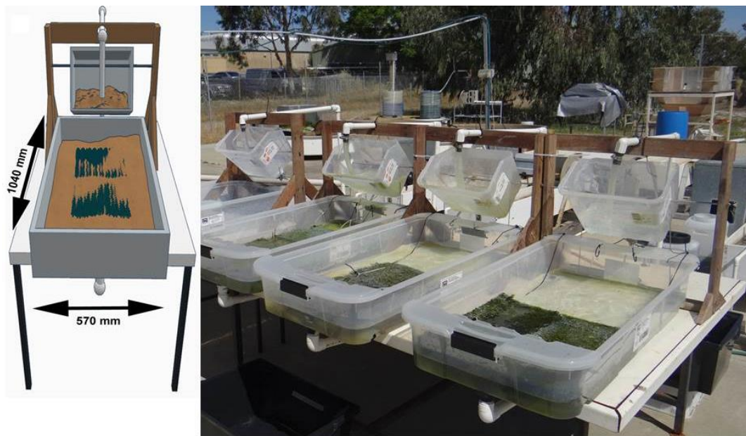
Figure 8. Schematic of the tipping bucket system used for the cultivation of the macroalgae.
