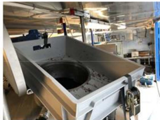
Figure 3: Transfer of bark to the tank using buckets (a 'platform' was constructed to omit spills)
