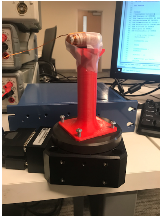
Figure 17: Sensor Mounted to Angular Displacement Control Motor
