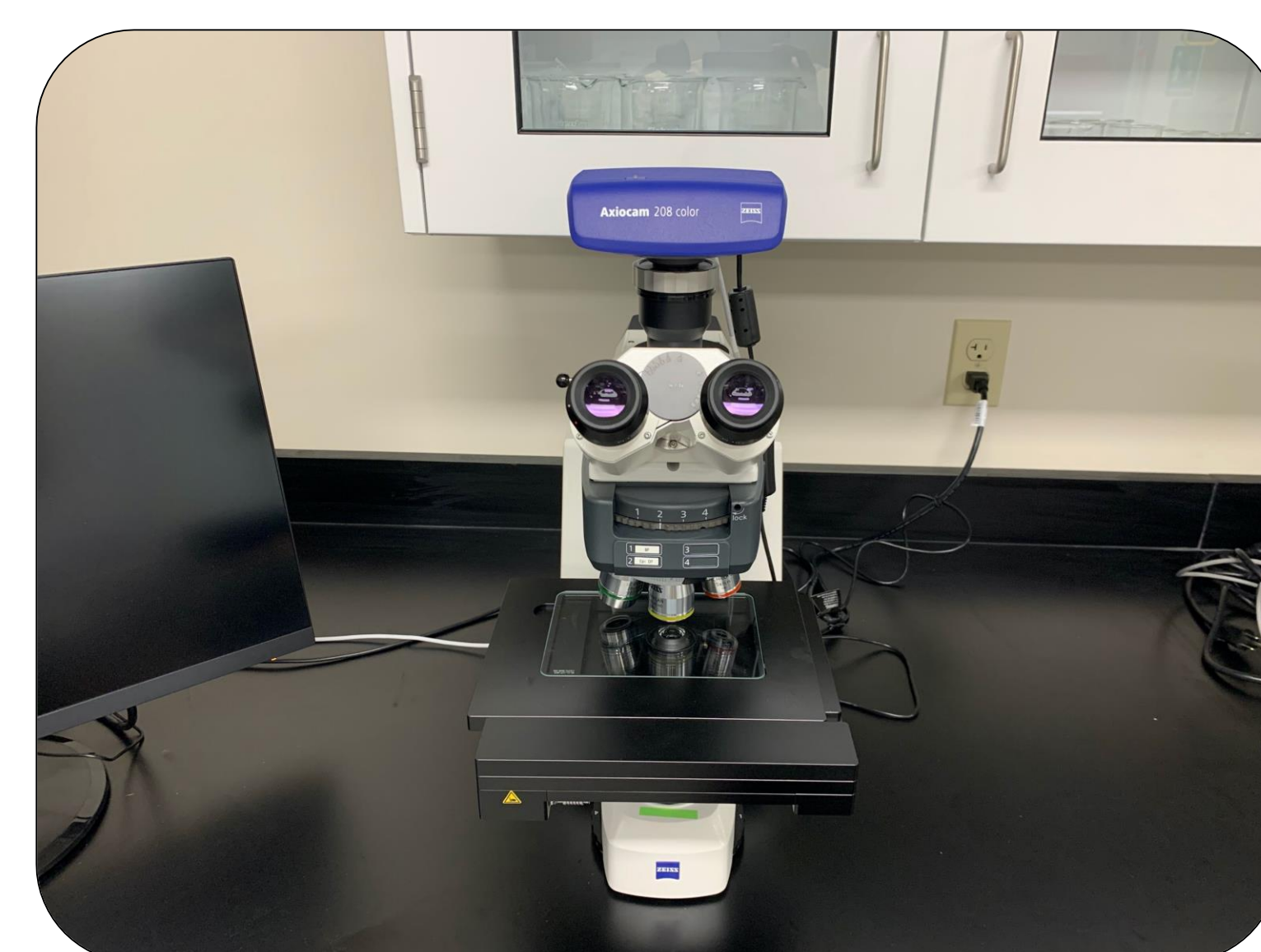
Figure 5: ZEISS Axioscope 7 compound microscope.
