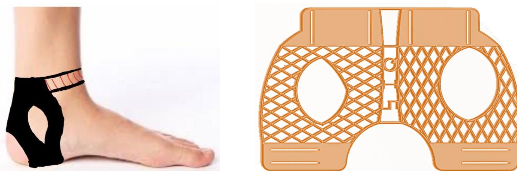
Figure 2: Concept of the ankle brace and SolidWorks CAD file of the first prototype.
