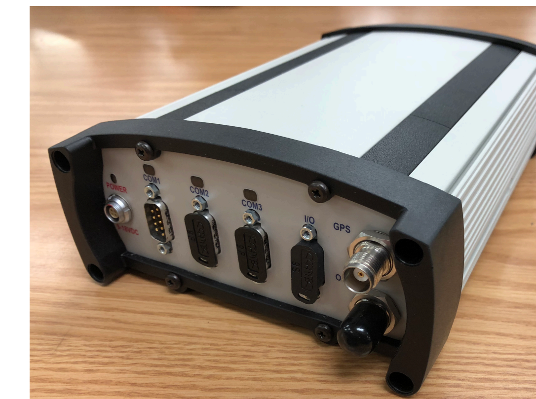
Figure 2: NovAtel GPStation-6 GNSS Ionospheric Scintillation Receiver
