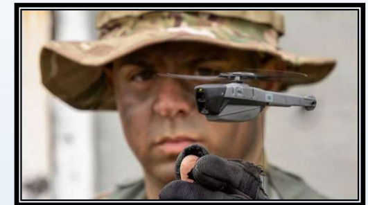
Figure 3. A Soldier with the (sUAS) Black Hornet Airborne Personal Reconnaissance System (PRS) by FLIR [10].
