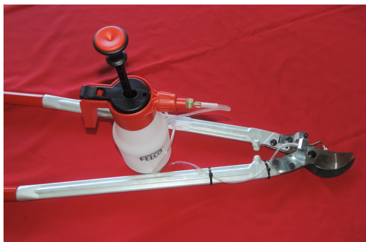
Modified pruning shears to be used on banana and plantain farms for control of YSD. (Photo: CELOS)
