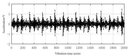
Fig. 7. Vibration data (0.18 mm inner ring fault size)
