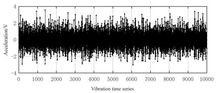
**Fig. 10.** Vibration data (0.72 mm inner ring fault size)
