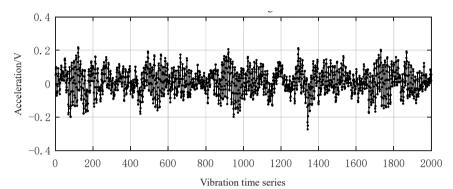
Fig. 6. Vibration data (normal bearing)
