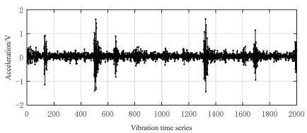
Fig. 8. Vibration data (0.36 mm inner ring fault size)
