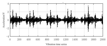
Fig. 9. Vibration data (0.54 mm inner ring fault size)
