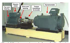
Fig. 4. Vibration experiment platform of rolling bearing
