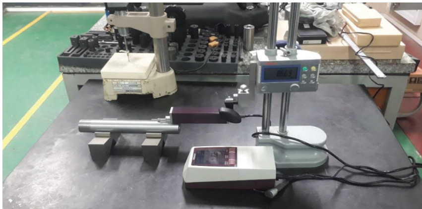
Fig. 2. Surface roughness measurement setup
