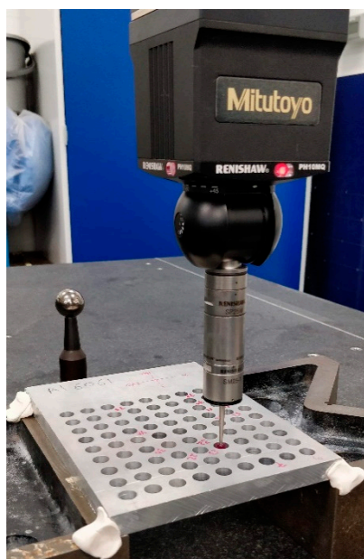
Figure 2. Al6061 workpiece setup inside the CMM machine.
