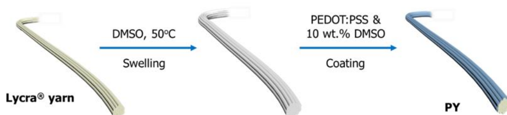
Figure 3.4 Schematic illustration of the 2-step swelling/coating fabrication procedure for the PEDOT:PSS coated Lycra® yarn (PY).
