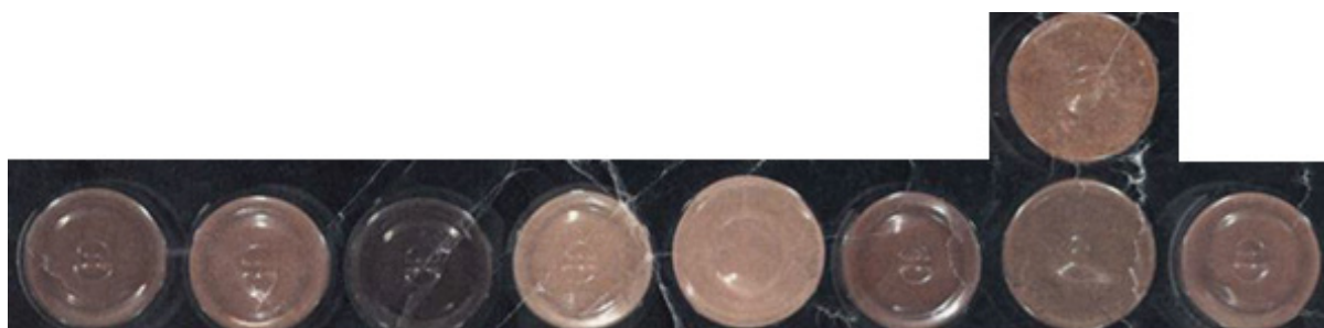
Picture 4-1. Illustration of how different the appearance (quality) of NOM samples (freeze-dried) can be among different watersheds. The lower row represents autumn isolates (photographed in scintillating glasses) of NOM from eight different watersheds at Nordic/Boreal sites, comparable to the NOMiNOR sites. Watershed second from the right has also been sampled during spring (top row), visualizing a difference in NOM quality during the season. Isolates are taken from the NOMiNIC-project (see Vogt 2001).
