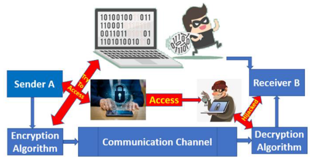
FIGURE 12. Plaintext Attack, on which the attacker tries to recover original data from chunk of known data.
