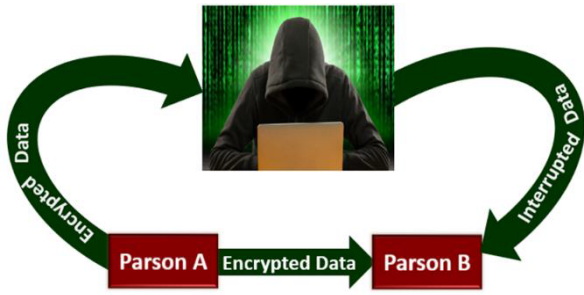
FIGURE 10. A man-in-middle attack disturbs the smooth transmission of data and secretly get the original data.
