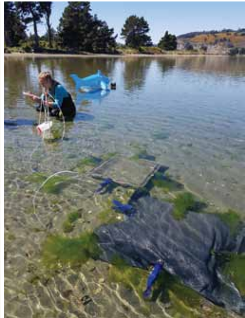
Figure 2. The paired light and dark chambers used to measure ecosystem functions like nutrient and oxygen flux in the field, in this case Blueskin Bay, Otago. Photograph: Candida Savage.
