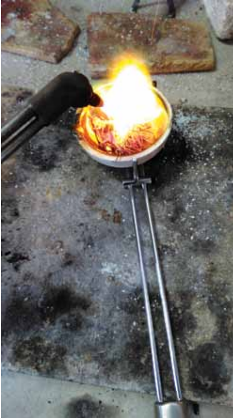
Figure 3. Melting copper and fine silver together to make alloys.
