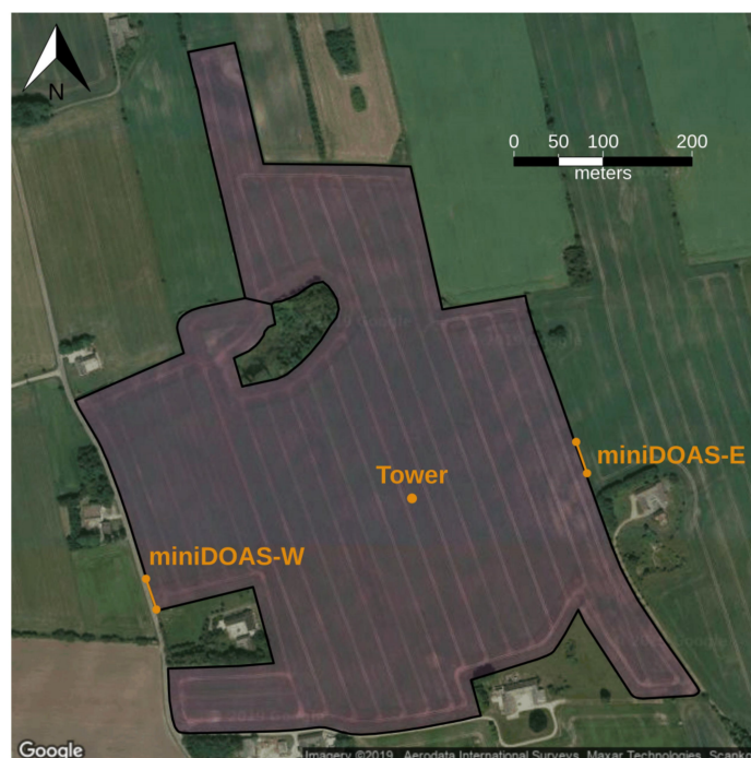
Figure 1. Overview of the field and measurement location on the field. The colored area is the 26-ha field where slurry was applied. MD-W and MD-E are the differential optical absorption spectroscopy (miniDOAS) located west and east, respectively, the tower includes the micrometeorological measurements and point concentration measurement of ammonia ( \text{NH}_3 ) with cavity ring-down spectroscopy (CRDS).
