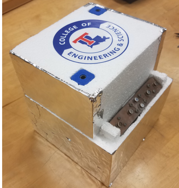
The Louisiana Tech team's balloon payload is shown prior to final launch preparations, with an array of UV sensors visible on the right hand face.
