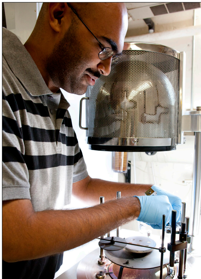
Bobby Mathew, post doc, prepares a thermal evaporator for depositing a thin layer of aluminum on silicon wafers in the Nanotechnology Lab
