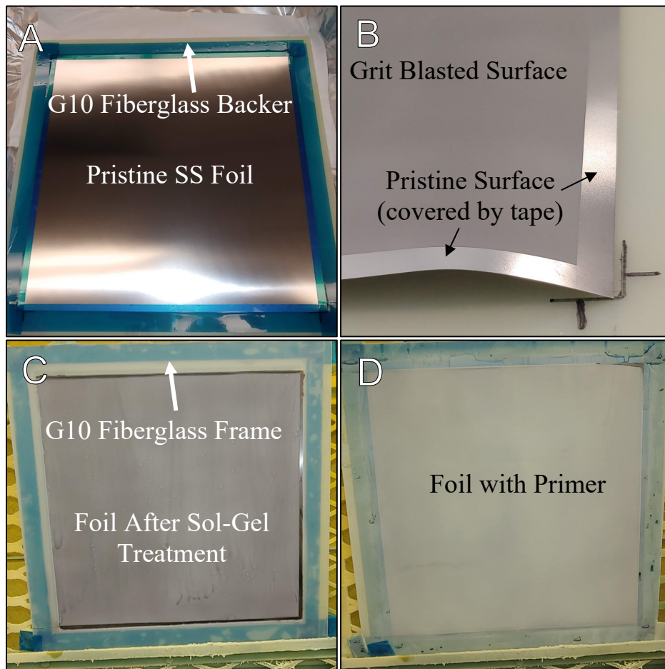
Figure 44: Stainless Steel Foil Preparation A) After Cleaning B) After Media Blasting C) After Sol-Gel Solution D) after Priming
