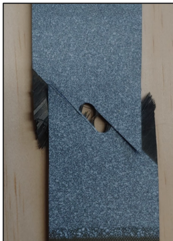
Figure 79: Expected Failure in 45° Ply
