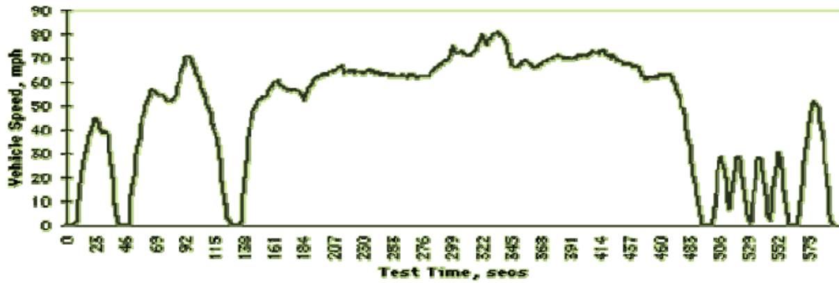
Figure 5. US 06 - Supplemental FTP Driving Cycle (31)
