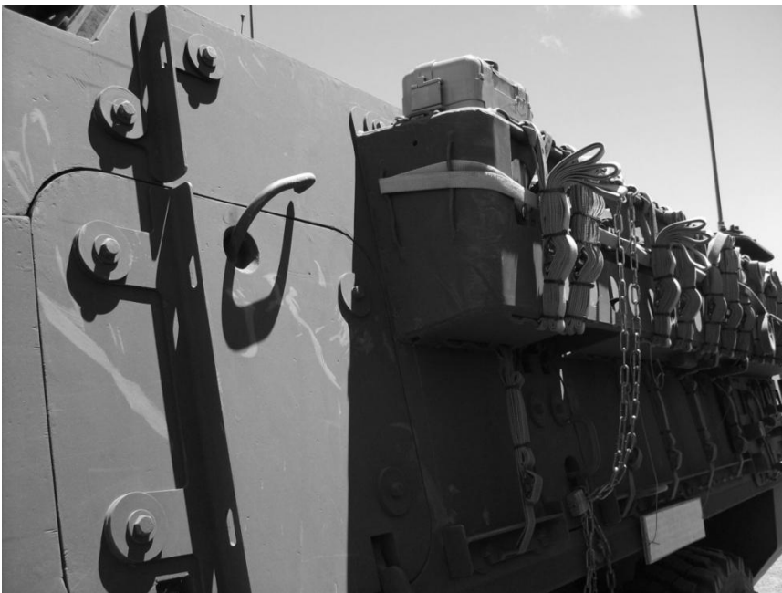
Figure 4-5: VTS mounted on a Stryker during post transformation
