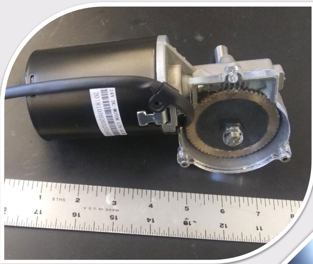
Figure 2: The two motors used to point the dish required replacement.
