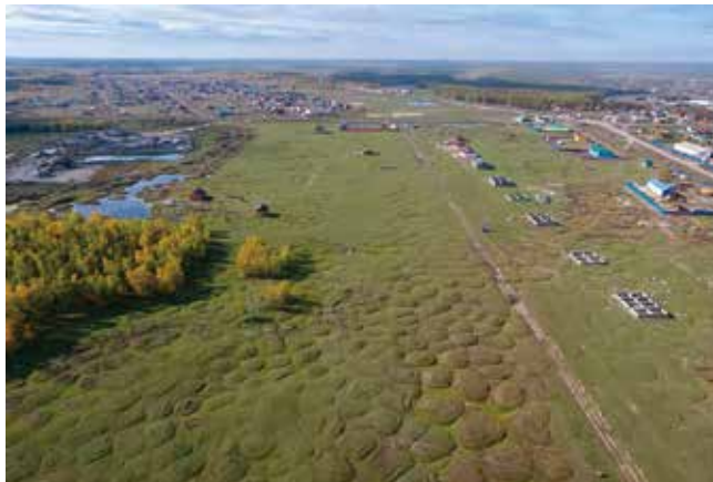
Fig. 1-1: Underground soil (former runway) affected by permafrost thaw in the village of Churapcha (photo by Y. Iijima, 2017).
