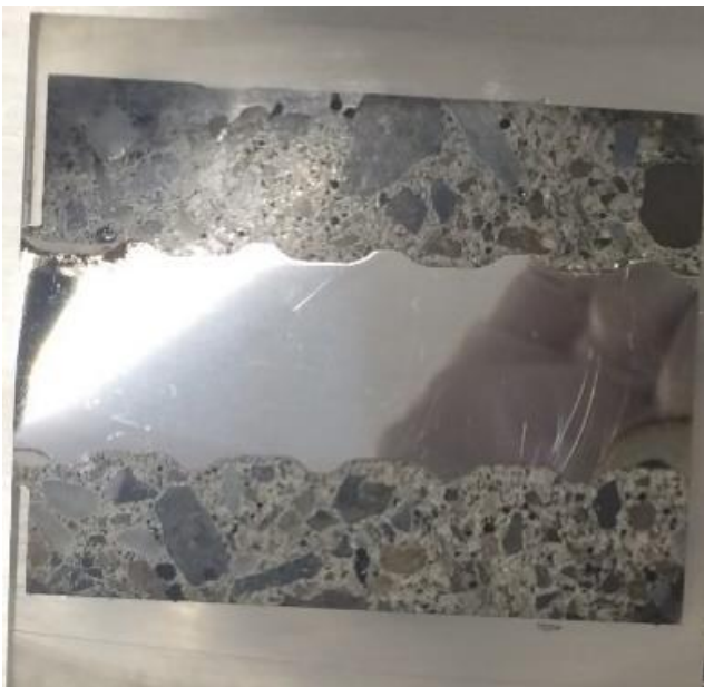
Fig. 3. Sample prepared for SEM-EDS observation on non-corroded steel specimen.
